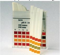
The test strips contain indicator dyes that are covalently bound to the reagent papers and then adhered to plastic strips. Contamination of the solution is therefore prevented even in strong alkaline solutions or from long immersion in weak buffered solution.
